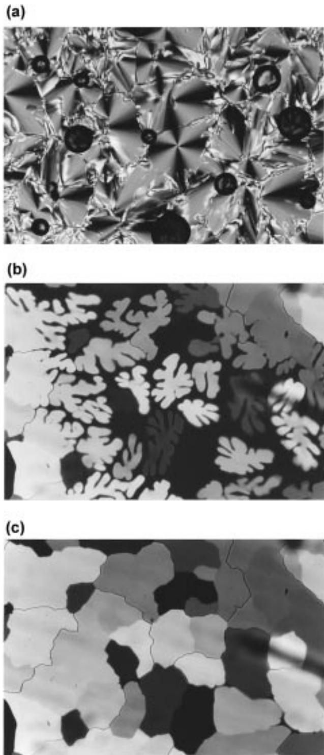
**Figure 4.** Optical photomicrographs of the mesophases of compound **1c** (crossed polarizers). (a) Spherulitic texture of the Col<sub>1</sub> phase at 39 °C obtained by cooling from the S<sub>A</sub> phase. (b) Fern-like texture at  $T = 87$  °C of the lyotropic Col<sub>2</sub> phase of the water-saturated sample as obtained on cooling from the isotropic state. (c) Mosaic-like texture of the Col<sub>2</sub> phase at  $T = 83$  °C.
