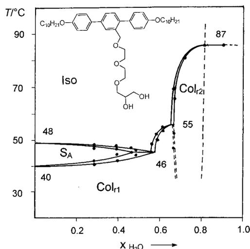
**Figure 2.** Binary phase diagram of compound **1c** with water.<sup>6</sup>
