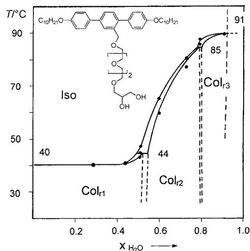
**Figure 5.** Binary phase diagram of compound **1d** with water.
