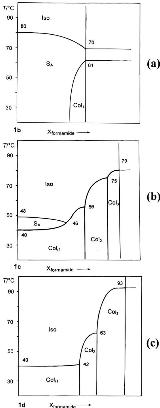
**Figure 6.** Simplified principal phase diagrams of compounds **1b–d** with formamide as obtained by investigation of the contact regions between crossed polarizers. Col<sub>1</sub> = columnar mesophase with spherulitic texture; Col<sub>2</sub> = columnar mesophase with mosaic-like texture; Col<sub>3</sub> = columnar mesophase with spherulitic texture.<sup>8</sup>
