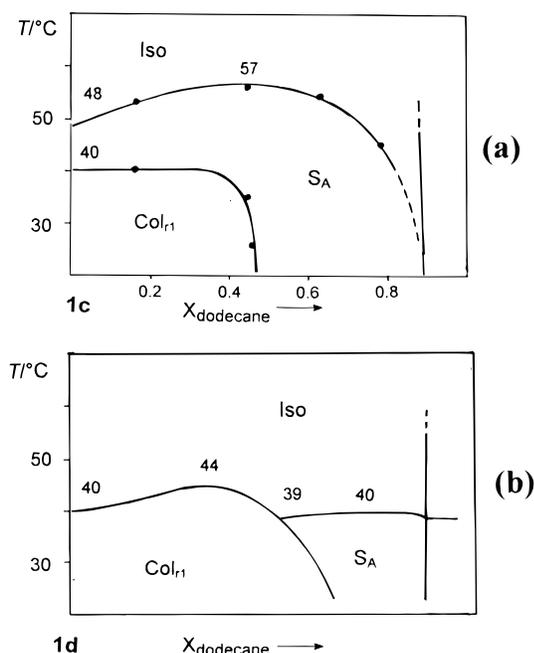
**Figure 8.** Simplified phase diagrams of compounds **1c,d** with dodecane.<sup>6</sup>
