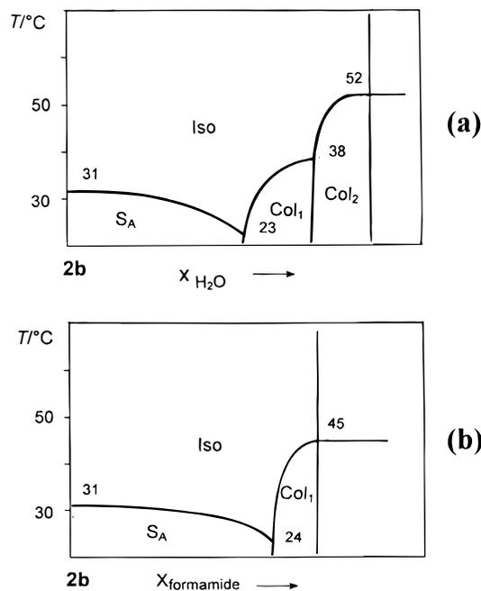
**Figure 7.** Simplified principal phase diagrams of compound **2b** (a) with water and (b) with formamide (Col<sub>1</sub> = columnar mesophase with spherulitic texture and Col<sub>2</sub> = columnar mesophase with mosaic texture).<sup>8</sup>
