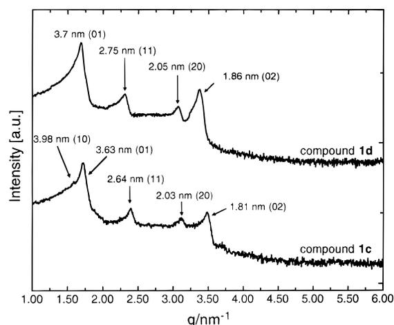
**Figure 3.** Small-angle region of the X-ray scattering diagrams of the lyotropic mesophase of the water-saturated sample of compound **1c** at  $80^\circ\text{C}$  ( $Col_{r2}$ ) and of the lyotropic mesophase of the water-saturated sample of compound **1d** at  $60^\circ\text{C}$  ( $Col_{r3}$ ).
